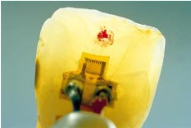
**Fig. 12.** Photomicrograph of tooth specimen 3 (original magnification,  $\times 3$ ) under transillumination, at end of trial. Multiple cracks are visible on palatal surface. One of these has propagated mesiodistally under strain gauge G1, explaining unusual and extremely intense signal given by this gauge (see Fig. 7).
