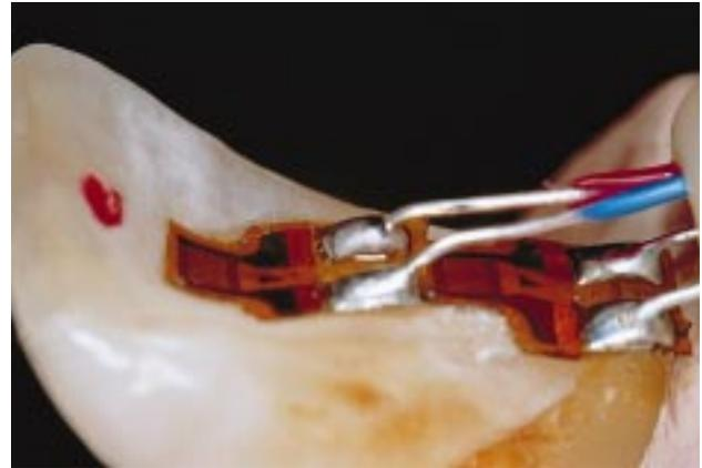
**Fig. 3.** Detailed view of specimen after placement of strain gauges. Axis of gauges follows longitudinal axis of tooth. Load point is marked in red.
